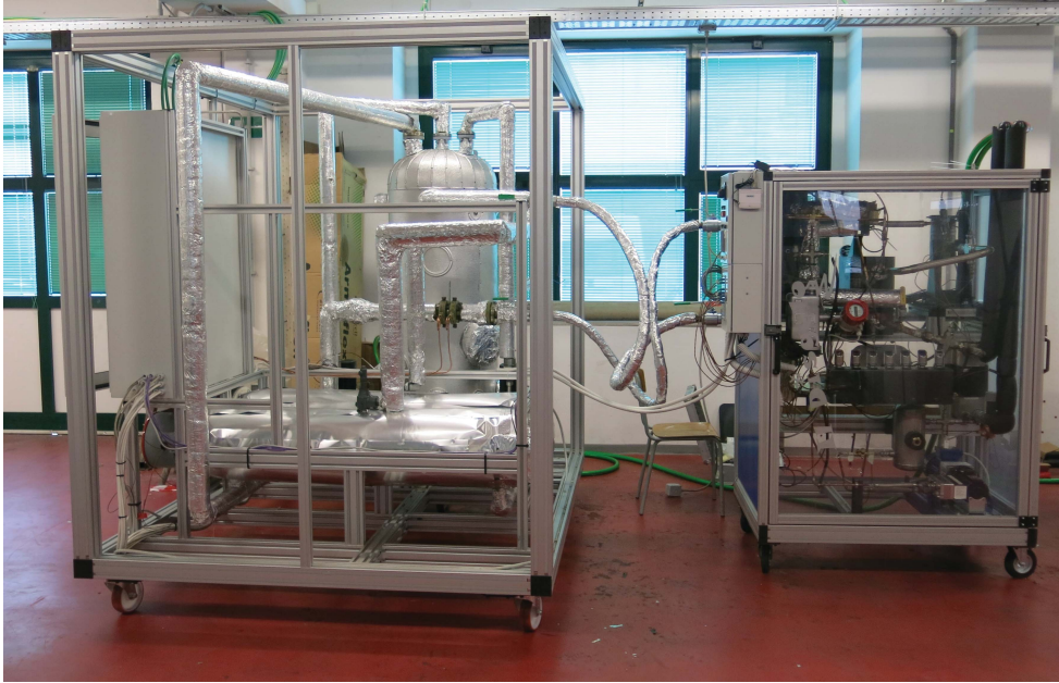
Figure 4.2: the ORC test facility at the University of Trieste.
