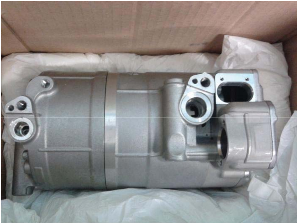
Figure 4.5: the scroll expander installed in the lab facility.
