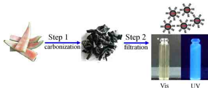
Figure 66: Schematic illustration of the synthesis of water-soluble fluorescent C-dots from watermelon peel [656].
