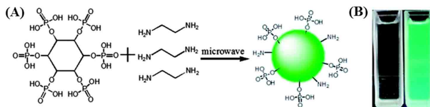
Figure 70: (A) Schematic diagram for synthesizing green C-dots. (B) Emission under daylight and 365 nm ultraviolet excitation [664].
