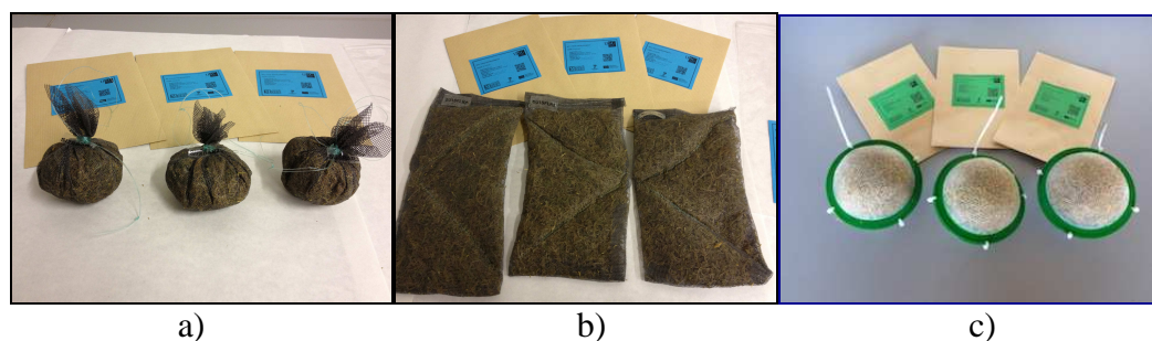
Figure 2. Different shapes of moss bags tested. a) Rounded; b) Flat; c) Mossphere.
