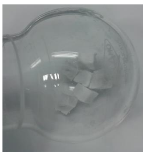
Figure 15. Final appearance of the AMG0.2 samples once they have been freeze-dried.
