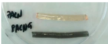
Figure 15. Digital picture of the semi-IPNs synthesised by following the Strategy 1: without graphene ( PACN ) and with graphene (0.2 mg/ml) ( PACNG ).
