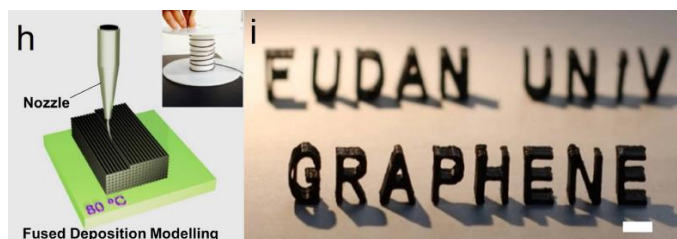
Figure 11. Schematic illustration of fused deposition modelling 3D printing process (inset is the graphene-based filament) and 3D printed model. Scale bar : 1cm. 68
