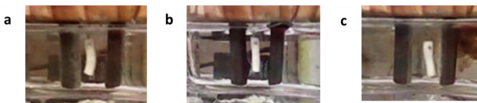
Figure 8. Digital pictures of the bending behaviour by the Blank a) after 1 minute of electric field application, b) without any electric field application, thus the sample is on a vertical position, c) after 1 minute of electric field application changing the current direction.
