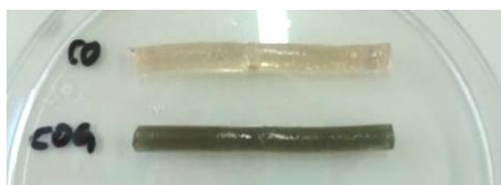
Figure 13. Digital picture of both copolymers hydrogels: without graphene ( CO ) and with graphene (0.2 mg/ml) ( COG ).
