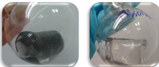
Figure 11. Appearance of AMG0.2 after having absorbed water (left) and AM after having absorbed the graphene dispersion (right).
