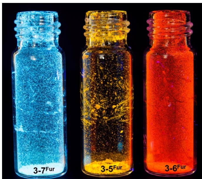
Figure 3.4.25 Photographs of fluorescent powders of compounds 3-7^{\text{Fur}} , 3-5^{\text{Fur}} and 3-6^{\text{Fur}} upon illumination with UV light (365 nm)
