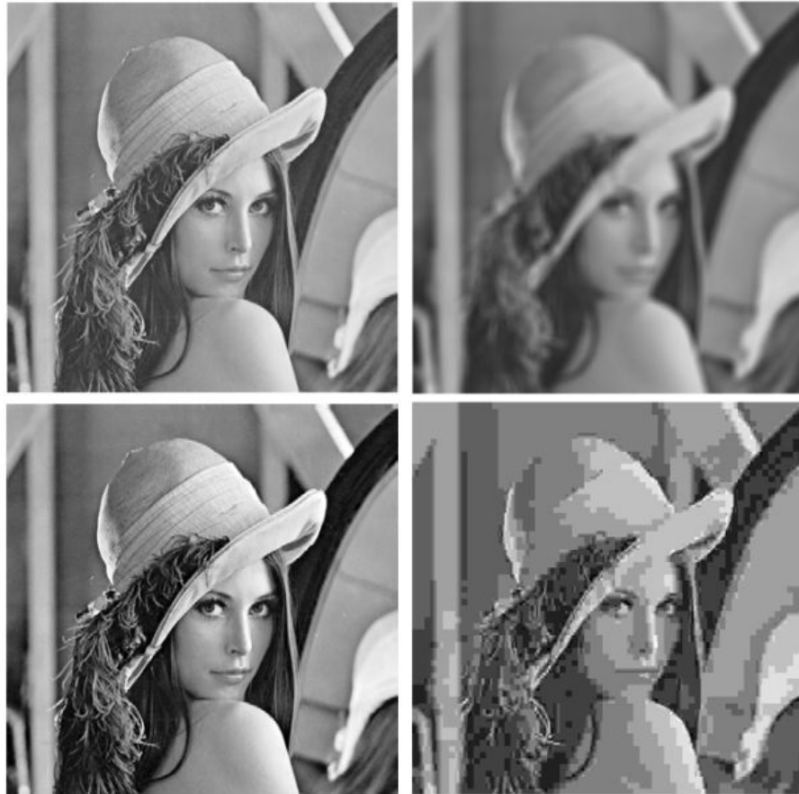
FIGURE 1.2: Images with 4 different type of distortions. Top-left: MSE=225, SSIM=0.99; top-right: MSE=225, SSIM=0.35; bottom-left: MSE=225, SSIM=0.94; bottom-right: MSE=225, SSIM=0.29 [22,Ch.41].
