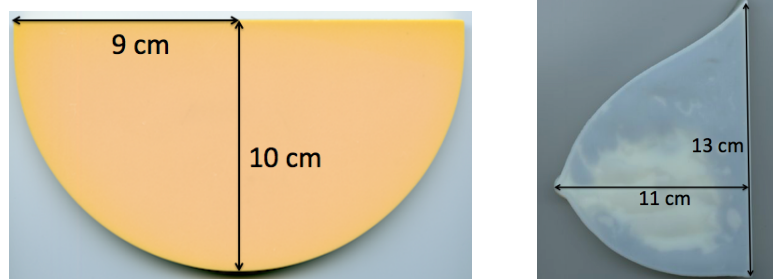
Figure 5.4: On the left side a slice of the 50%-50% homogeneous phantom produced by CIRS. On the right side a slice of the heterogeneous phantom: the whiter inner part is the glandular part (courtesy of Ioannis Sechopoulos).
