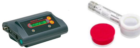
Figure 5.2: Dose monitoring system (left side) and mammography probe of the RADCAL chamber (right side).
