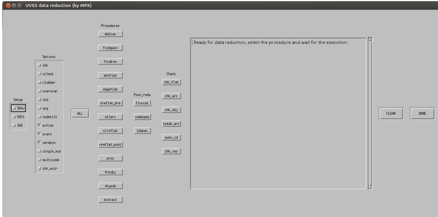
Figure 3.3: Graphical User Interface of the new pipeline (UVES mode in this example). The layout is very simple and allows to perform each one of the reduction step (in the Procedures column) interactively checking the results in real time selecting the chk options, or at the end of the execution with the procedures in the Check column. The user has also the possibility to perform automatically all the steps in one take using the “ ALL ” button.
