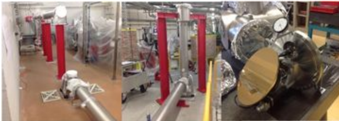
Figure 6 Transport pipes and vacuum chambers of the TeraFERMI beamline inside the safety hutch (left) and undulator hall (center). Right: plane mirror mounted in its holder and ready to be installed.
