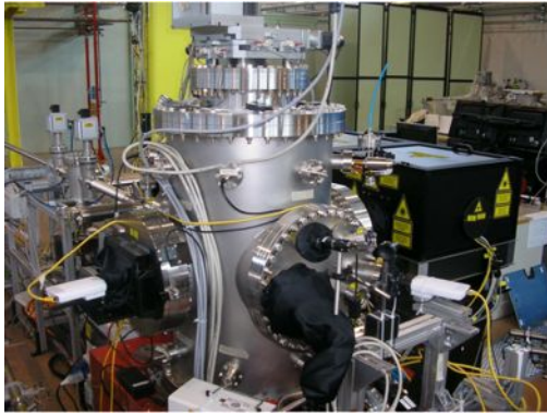
Figure 14 Left: External view of the main EIS-TIMEX chamber. On the right one can distinguish the black box that protects the laser setup . Right: EIS-TIMEX end-station main experimental setup.
