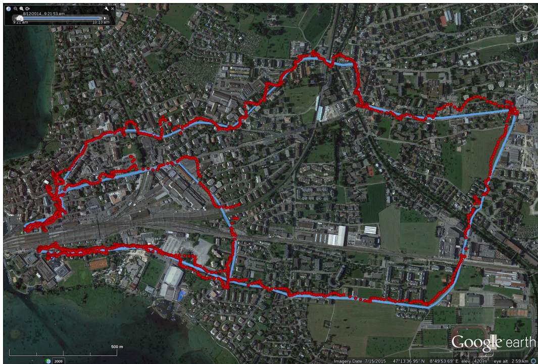
(a) Outdoor vehicular dataset. The red markers are the position solutions. The blue line is the ground truth.
