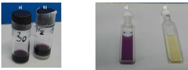
Figure S4.14 a) DPPH solution at t = 0 on empty vial; b) DPPH solution at t = 0 in contact with NCND-gel; c) DPPH solution unexposed to gel phase at t = 1 h; d) DPPH solution exposed to gel phase at t = 1 h.
