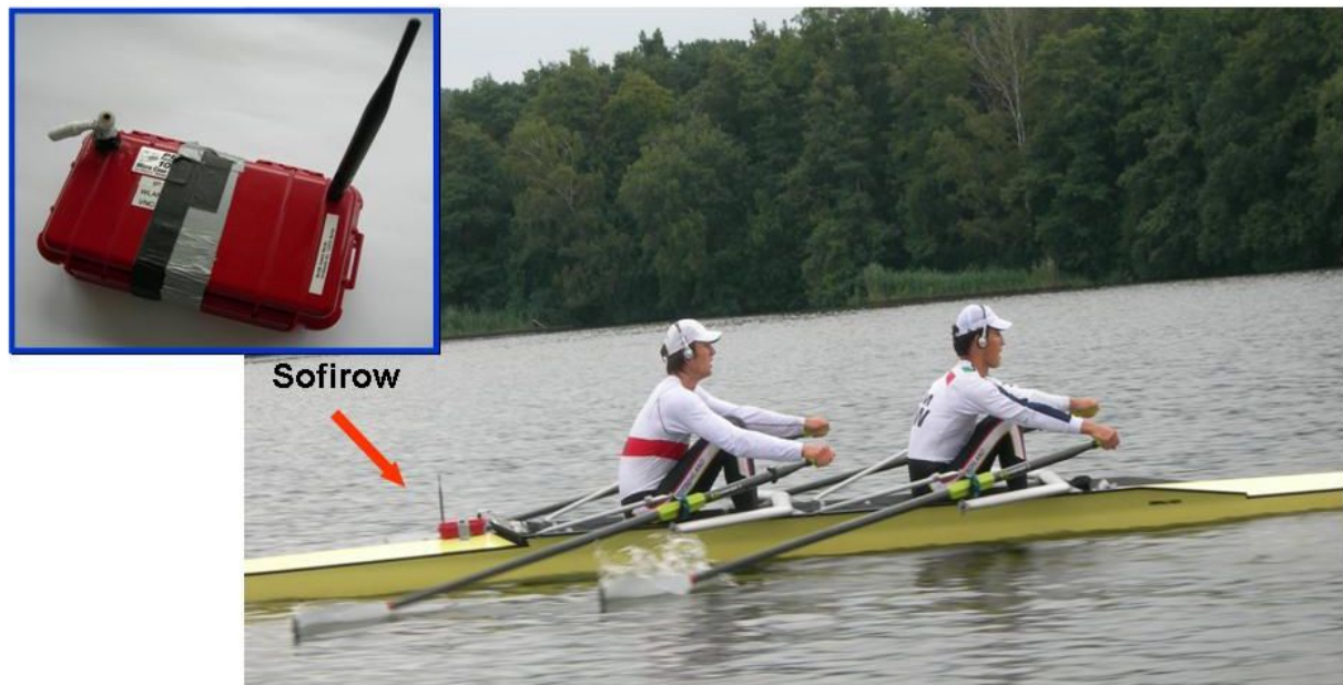
Figure 2. The sonification device used by Schaffert and colleagues (2011; image from Schaffert, Mattes and Effenberg, 2010, p. 32). The auditory feedback could have been delivered either via loudspeaker or via headphones (like in this example); moreover, the device could have been switched on and off by remote-control from the accompanying coaching boat.
