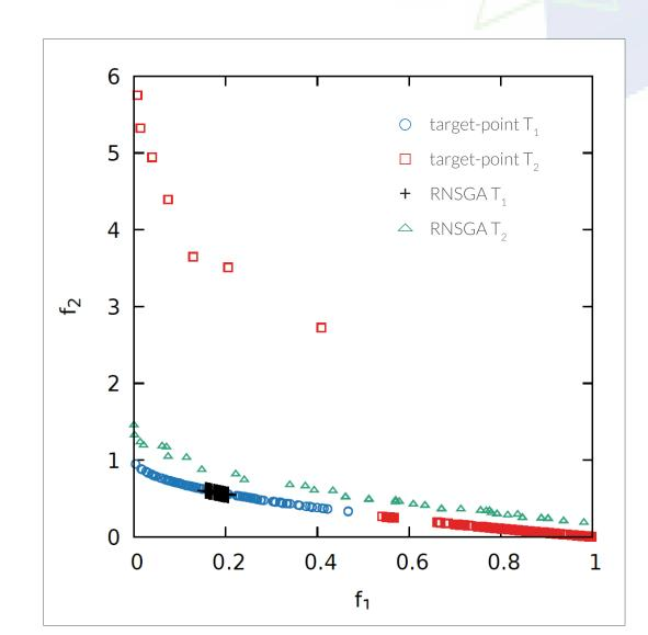
For each algorithm, two optimizations with target values  $T_1 = (0.2, 0.6)$  and T<sub>2</sub> (0.9, 0.1) very close to true Pareto front. Both algorithms are run for 100 generations starting from initial population of 50 random individuals.
