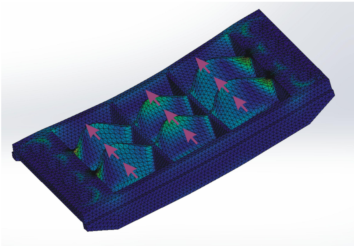
Figure 26: Forces perpendicular to the side surfaces of the retention cage housings to perform FEM analyses.
