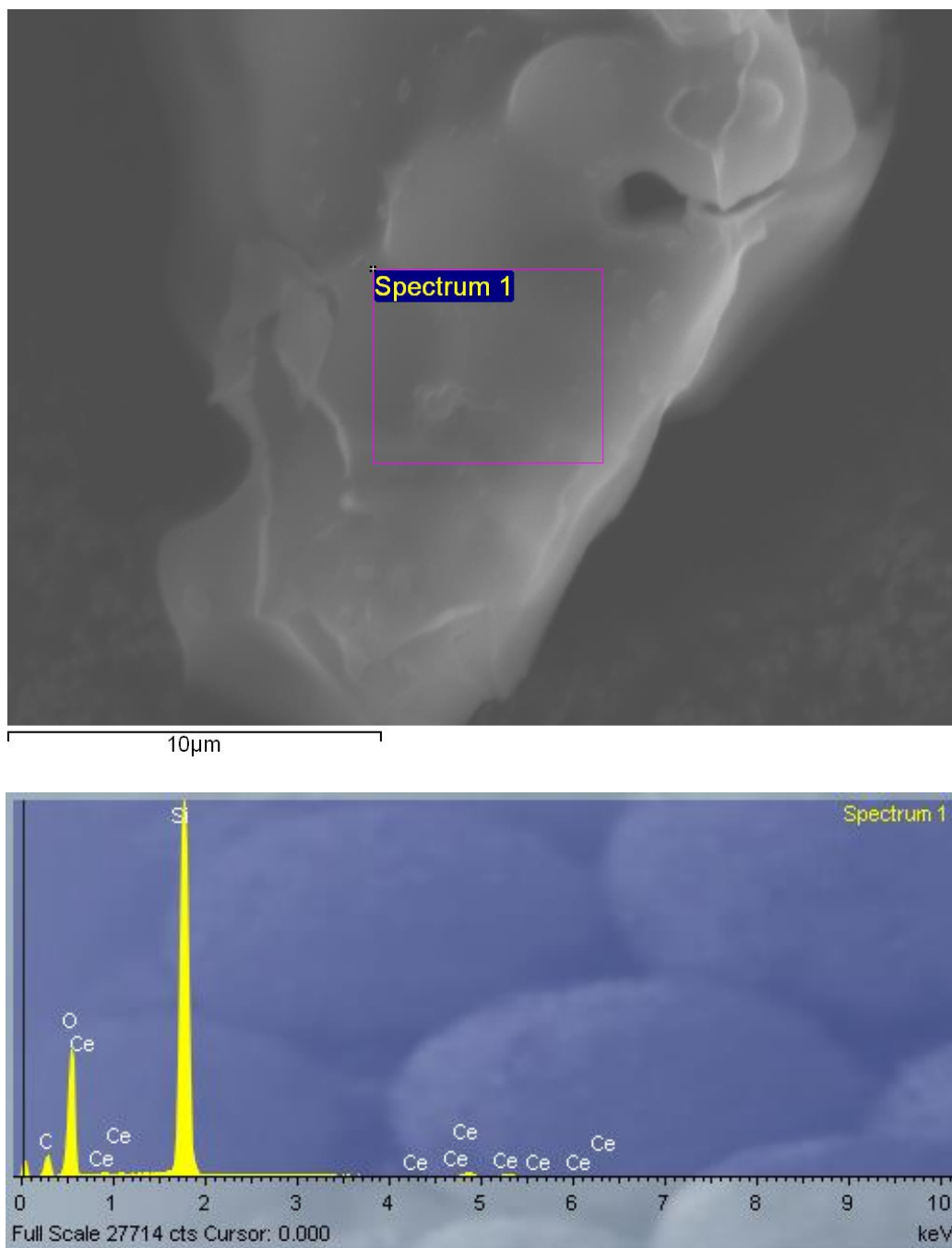
Fig S3. SEM image of and EDX spectrum obtained from the area indicated in the image for IMP_Pt/CeO 2 (10%)/H-SBA-16.
