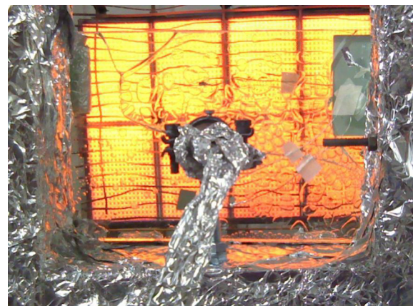
Fig. 14. Testing of a laminated glass panel exposed to a radiant heat flux, as reported in [131]. Note the bubbles forming in the interlayer, as it melts and evaporates.
