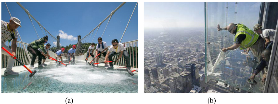
Fig. 4. Safe design of structural glass systems. (a) Robustness assessment of the 300 mm high 'Zhangjiajie' glass bridge in China; (b) glass failure at the 103rd floor of the Willis Tower in Chicago (photo: AP).
