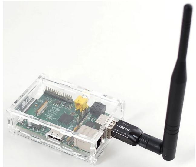
Fig. 2 – Hardware platform implementing the evil twin used in our experiments (the battery is omitted).
