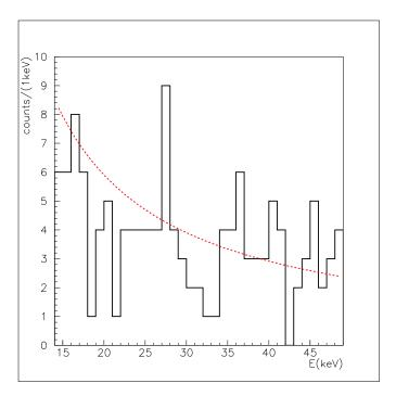
**Figure 1.** Fit of the X-ray emission spectrum measured by the IGEX experiment [19,20], using the theoretical fit function Equation (7). The black line corresponds to the experimental distribution; the red dashed line represents the fit. See the text for more details.
