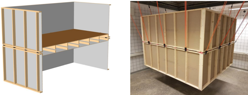
Figure 1: The experimental wooden building structure representing a part of a two-storey TVE building. To the left: a rendering of the correlated structure cut perpendicular to the wood beams and to the right: photograph of experimental setup.
