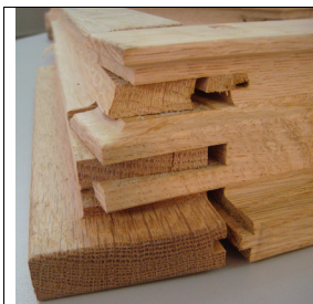
Fig 1. Tenon-mortise corner joint.
