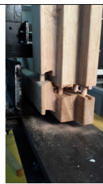
Fig 2 Dowel corner joint
