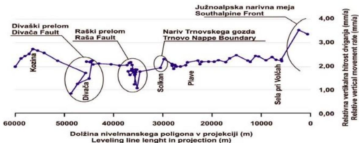
Figure 7: Relative vertical movement rate over a part of the active faults of the Dinaric strike slip system derived from levelling line (Rižnar et al. 2007). Clear changes are observed over so called Divača fault, Raša fault Trnovo Nappe thrust fault and Southern Alps thrust front. From earthquake activity only Raša
