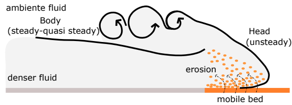
Figure 1.5: Schematic view of the bed material entrainment induced by gravity currents
