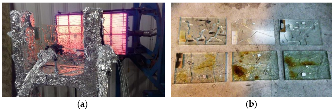
Figure 3. Thermal experiments on MG and LG specimens: (a) test setup (with an exposed LG sample) and (b) typical damage scenarios for the failed specimens, at the end of the radiant heating tests (Copyright © Dániel Honfi).
