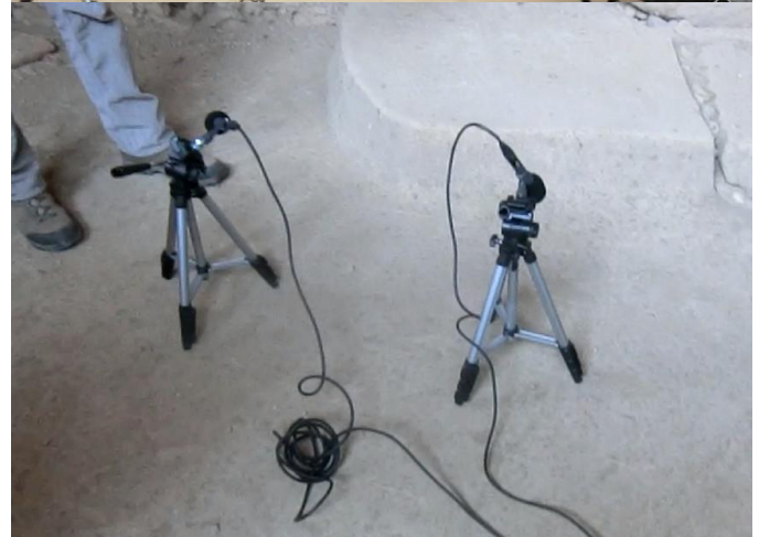
Figure 4. We placed the microphones close to the limestone floor near the base of pillar n.18, directed towards the floor.
