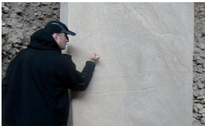
Figure 16. The maneuver to stimulate resonance of the pillar n.18 by a delicate tap of the fist.
