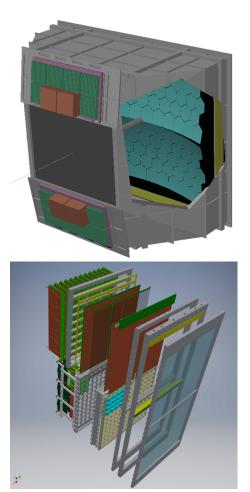
**Figure 1.** Artistic view of the COMPASS RICH-1 detector (left) and exploded view of the new PDs (right)
