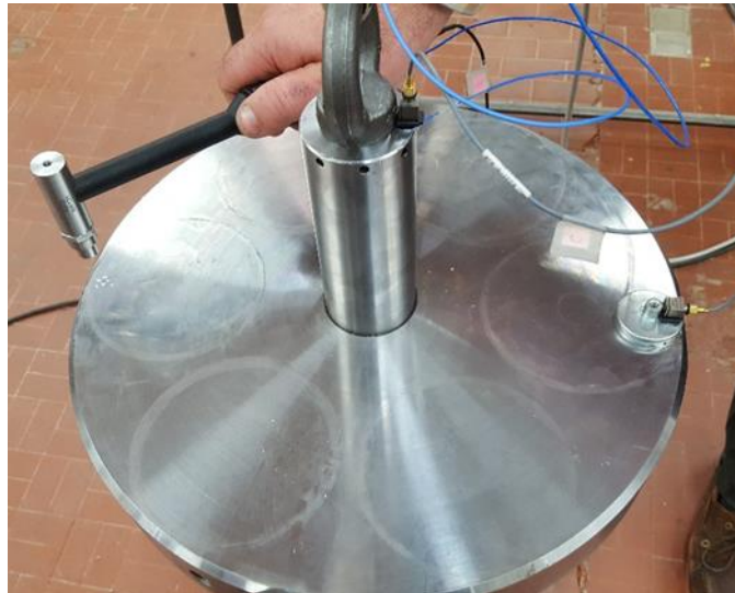
Figure 19: Suspended disk for its normal mode analysis
