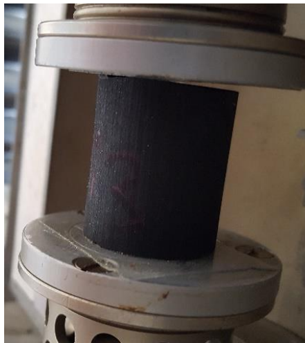
Figure 71: Contact issue for the sample
