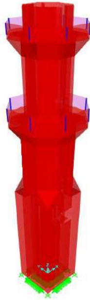
Fig. 5.13. Detailed finite element model of the minaret.
