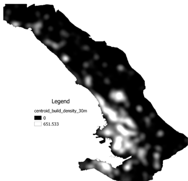
Figure 4. The building density map obtained by the application of the Kernel Density Estimation method to the centroid vector layer (Figure 3).
