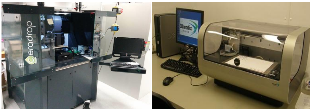
Fig 6.1: two types of high-resolution inkjet printers; left: CERADROP 3000. Right: Dimatix Fujifilm, DMP 2831.
