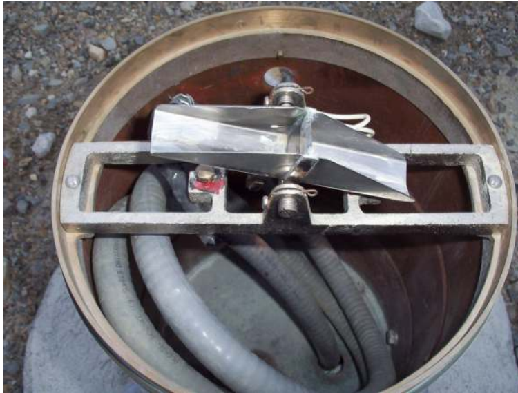
FIGURE 2.1: A tipping bucket rain gauge, the most common type of precipitation measuring instrument, with the buckets exposed.
