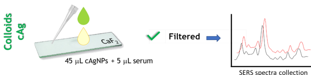
Figure 8.3 Sketch of the sample preparation for spectra collection.
