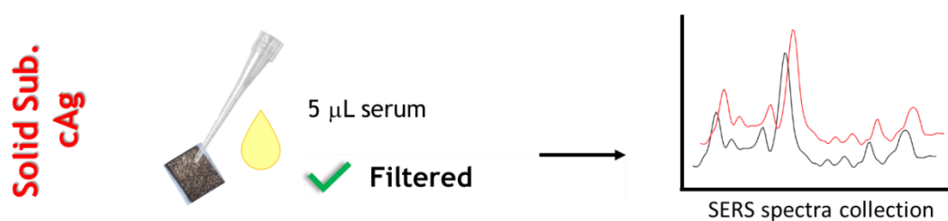
Figure 8.7 Sketch of the sample preparation for spectra collection.
