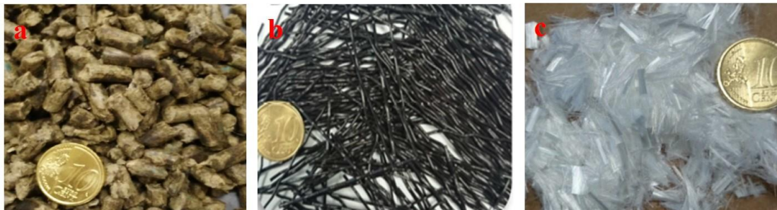
Figure 1. Fibre types: a) cellulose-glass fibre (C), b) structural fibre (S) and c) multifunctional fibre (M).
