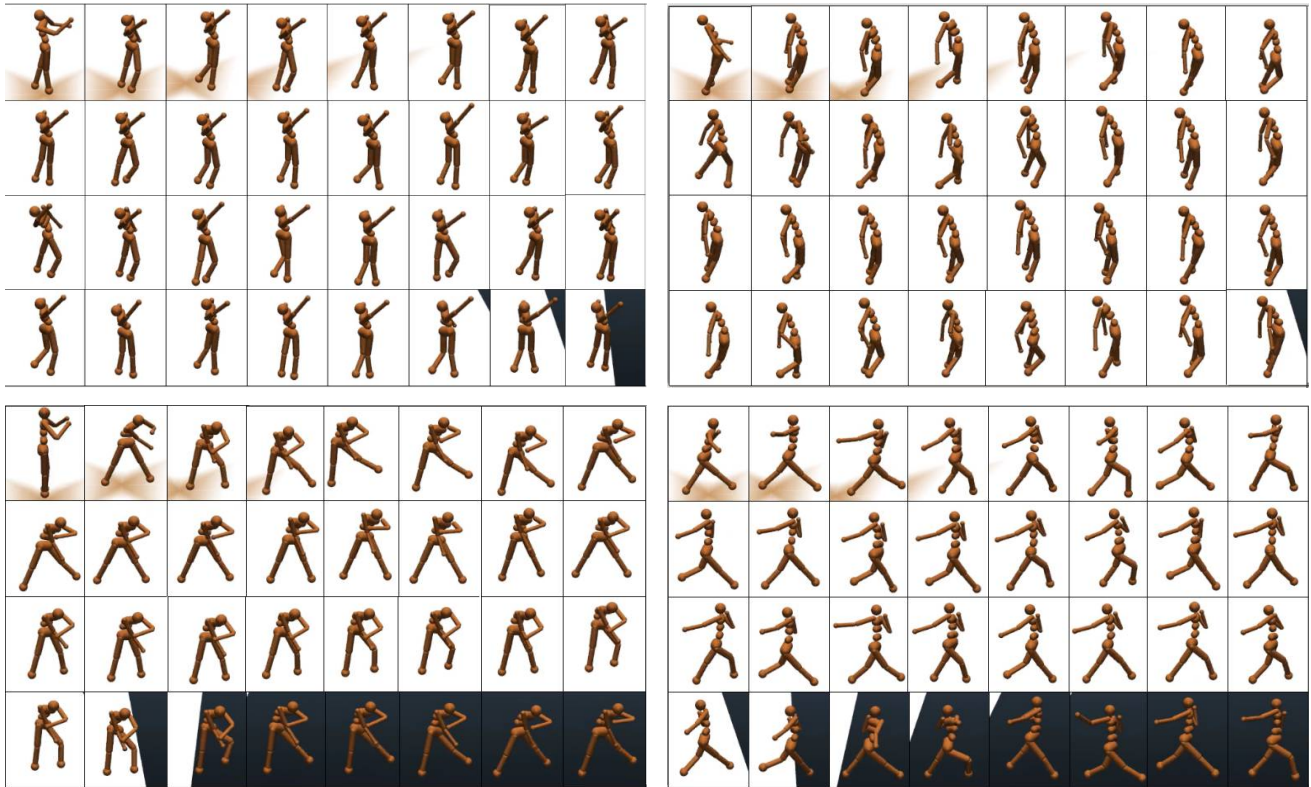
Figure 8: Gaits with noise = 0.4, from the controllers shown (without noise) in figure 5. Frame order is from left to right and top to bottom. In the default-runs gait (top-left) the biped shuffles by alternating its knees in a more erratic way than before. In the s500-runs gait (top-right) the biped still puts one leg in front of the other, but much more loosely. In the rp75-runs gait (bottom-left) the biped uses one arm for momentum and is not affected too heavily by the noise, only bending its back more. In the combo-runs gait (bottom-right) the biped shuffles on its knees with a wide stance, making more flailing motions than previously. (The darkness at the end of the figures occurs as the humanoids walk out of the range of the white floor texture.) Videos of these gaits can be found at https://github.com/KeeleBenJa/bipedal-methods .
