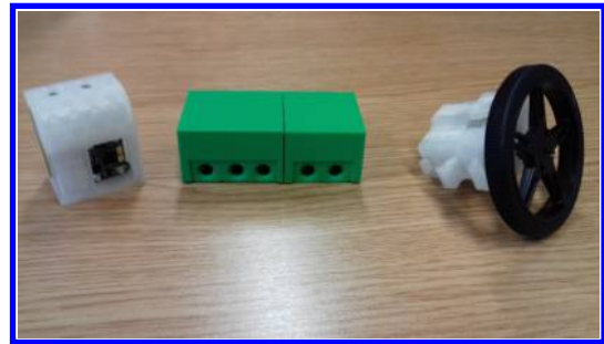
Figure 4: Prototype organs in the physical world. From left to right: a sensor organ, brain organ and wheel organ.
