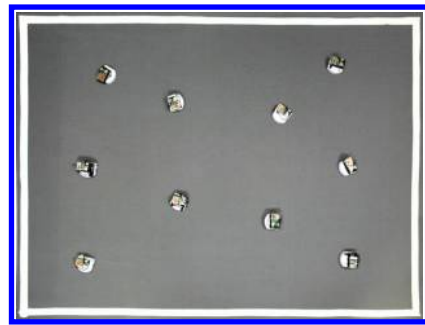
Figure 3: The 3.0 \times 2.5 m 2 arena is bound by a white line on the ground (duct tape) emulating virtual walls that can be detected by the robots’ ground sensors. N = 10 robots are initially placed in an evenly spaced grid.
