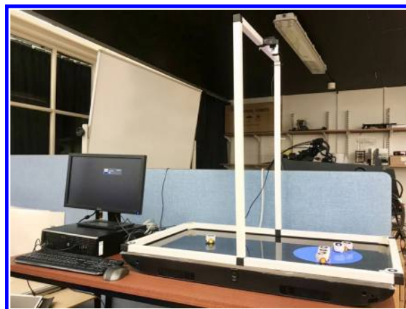
Figure 1: Artificial pheromone system including a horizontally placed LCD screen, overhead camera for tracking system and a computer.
