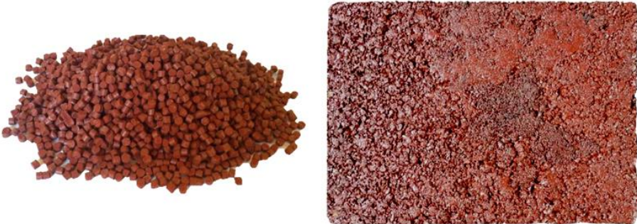
Figure 5.38. Red oxide-pigment (left) and BL(oxR) slab (right).
