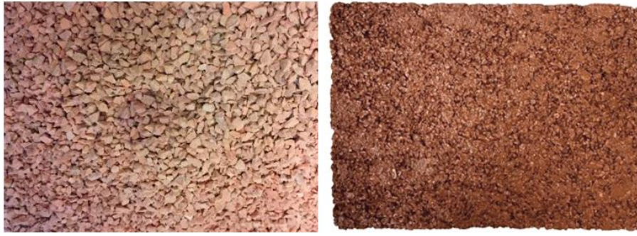
Figure 5.36. Coral-pink stone aggregate (left) and SP slab (right).
