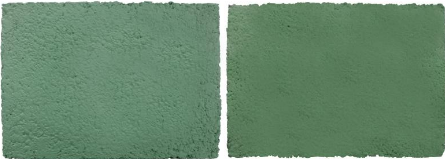
Figure 5.43. Green slabs painted with resin (left) or mortar (right).
