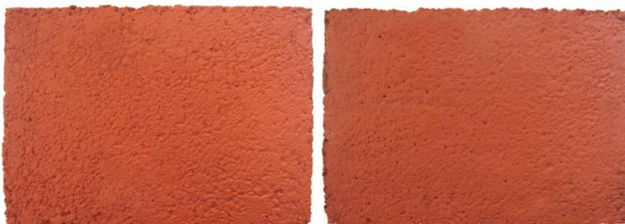
Figure 5.42. Red slabs painted with resin (left) or mortar (right).
