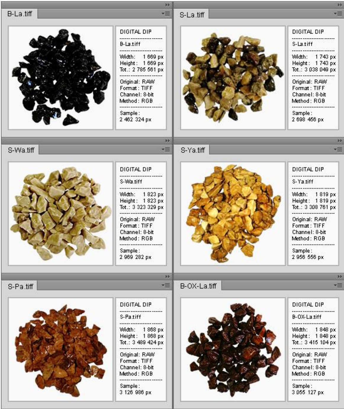
Figure 5.26. Example of stripping results: DIP output (original samples before AST).
