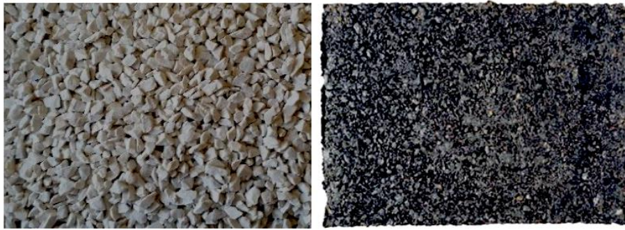
Figure 5.30. Limestone aggregate (left) and example of produced slab (BL mixture – right).
