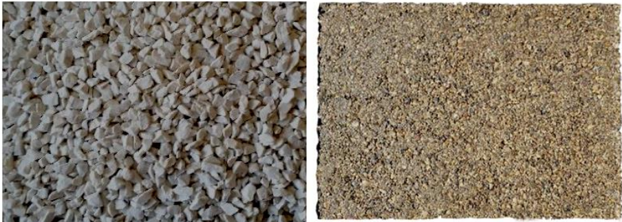
Figure 5.33. Limestone aggregate (left) and SL slab (right).
