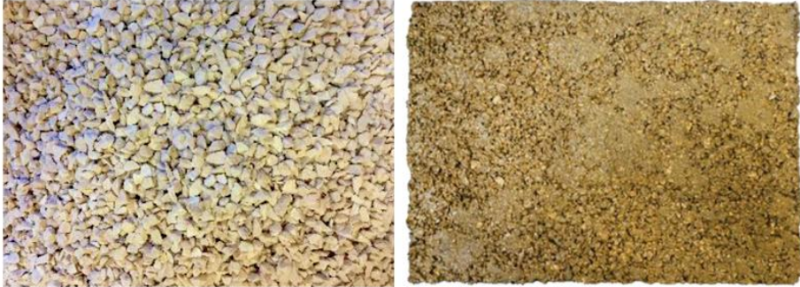
Figure 5.35. Yellow-Siena marble aggregate (left) and SY slab (right).
