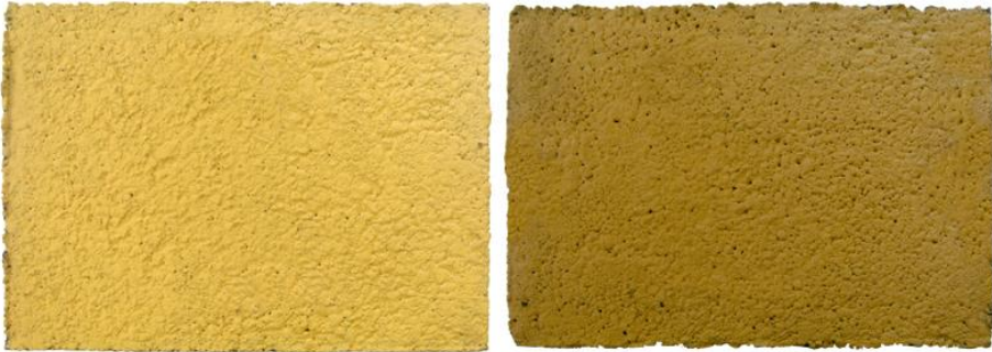
Figure 5.44. Yellow slabs painted with resin (left) or mortar (right).
