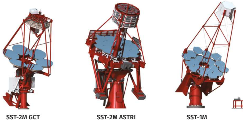
Figure 1.11: 3D models of the SSTs. The first two models use the Schwarzschild-Couder double mirror configuration while the SST-1M uses only a primary mirror.
