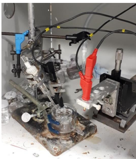
Figure 5.7 Picture showing the three-electrode glass cell employed to carry out the electrodeposition of gold.
