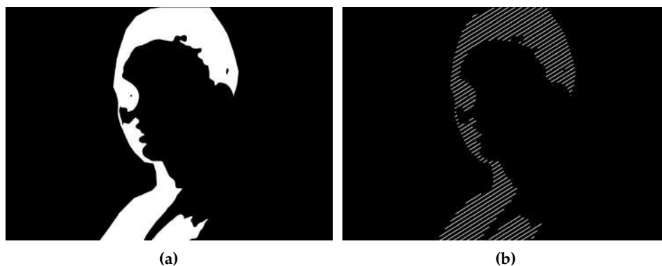
Figure 9. Marina low frequencies processing example: Layer 5, binary image, l_5 = 51 (a); processed layer (ang. 32^\circ , dist. 20px) (b).
