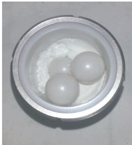
Figure 4.20: Example of the jar partially filled with the powder to be ground and with the milling media.
