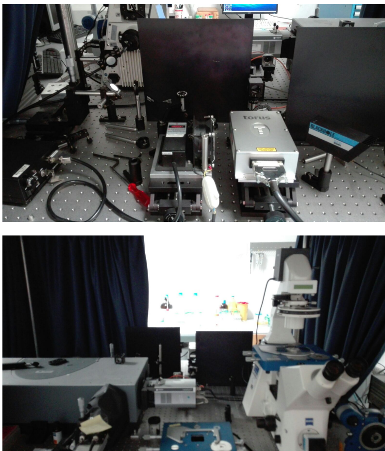
Figure 6.6: Experimental setup: the image on the top represents the irradiating laser and the bottom shows the sample holder and the microscope used for imaging.
