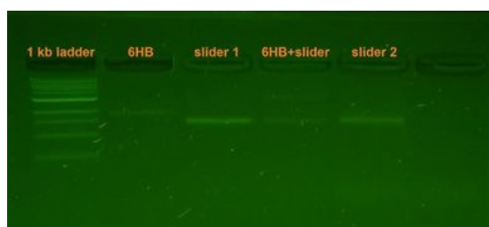
Figure 7.7: Gel electrophoresis analysis to check the correct assembly of the 6HBs and the slider origami.
