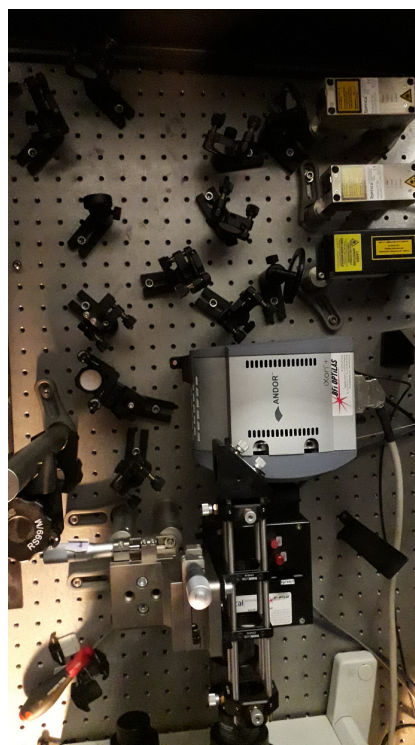
(b) Picture of the experimental FRET setup employed for our measurements.
