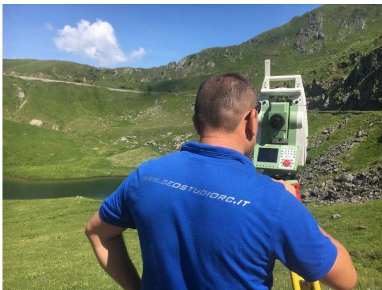
Figure 6. Total station (LeicaTS15) used to measure the network (photo: Paolo Pastorino).
