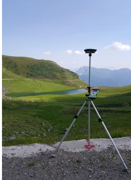
Figure 7. Location referencing with GNSS System Leica GS14 (photo: Paolo Pastorino).
