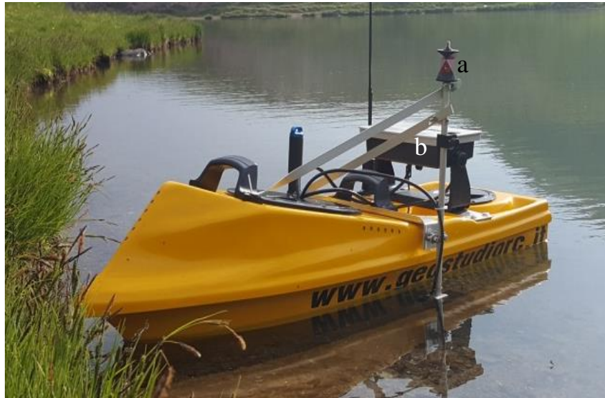
Figure 4. Equipped boat used for bathymetric survey. a) 360° Leica prism; b) Garmin Gpsmap 722XS (photo: Paolo Pastorino).
