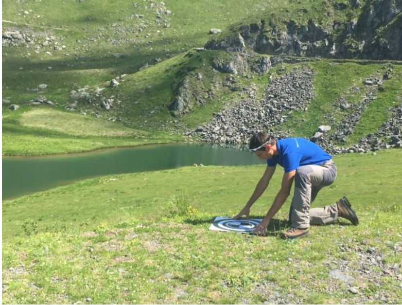
Figure 5. Positioning of photogrammetric cross-targets on the ground (photo: Paolo Pastorino).
