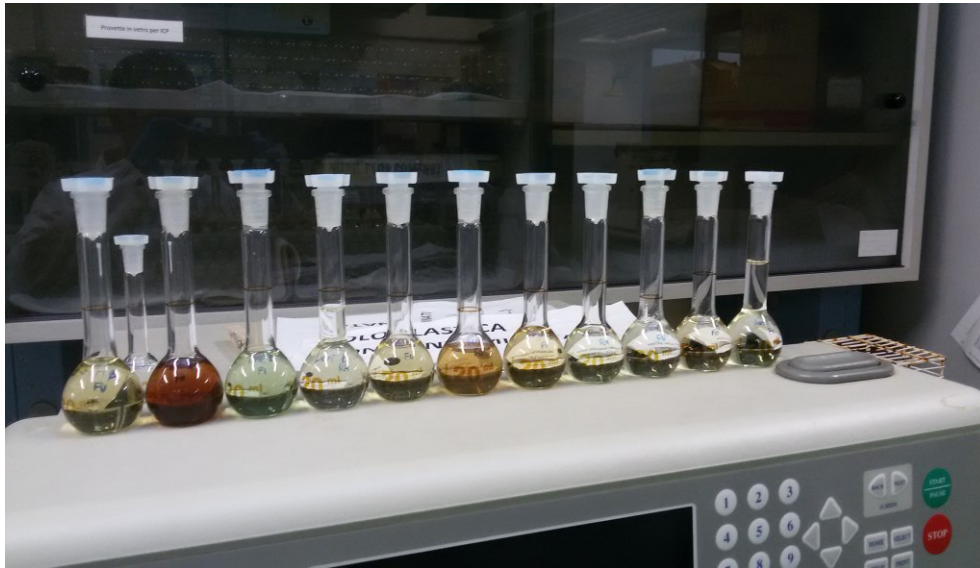
Figure 17: Samples in 20 mL flasks, where plant samples are transferred after acid digestion and before filtration.
