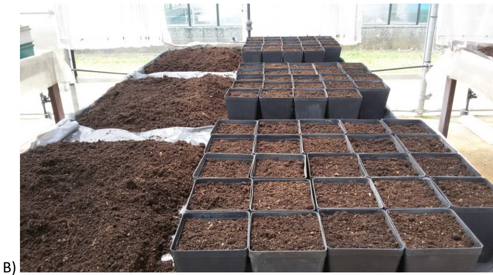
Figure 12: Pot soil experiment in the greenhouse: in image A), topsoil amended with n\text{CeO}_2 solutions (25 and 50 nm) at different concentrations (0, 2, 20, 200 \text{mg L}^{-1} ); in images B), topsoil put in pots and classified for treatments.
