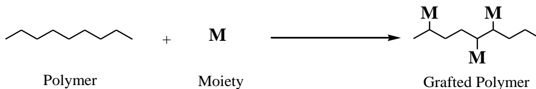
Figure 12.3: Schematic representation of grafting process.
