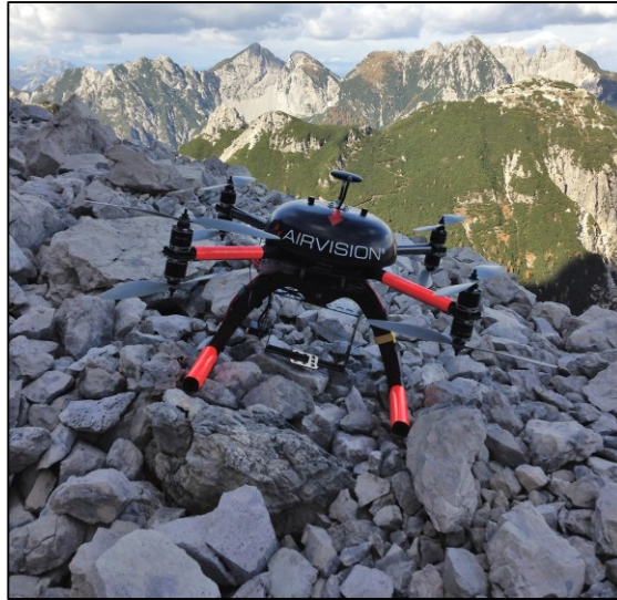
Figure 4.9: The 8-rotors UAV used for the surveys.
