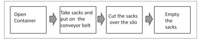
Figure 1 - Work process lay out
