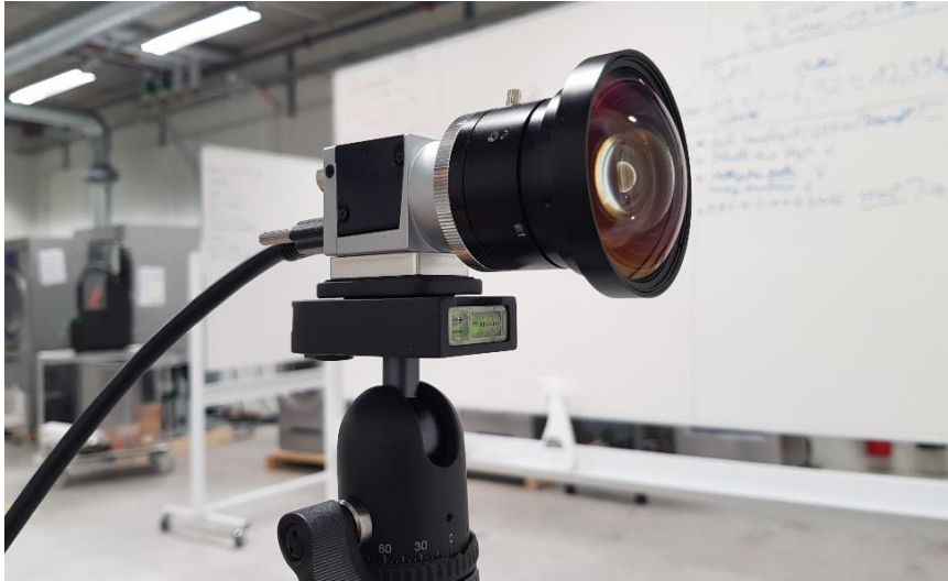
Figure 26. Industrial camera, coupled with a wide optic, used to acquire images for the automatic sorting system.
