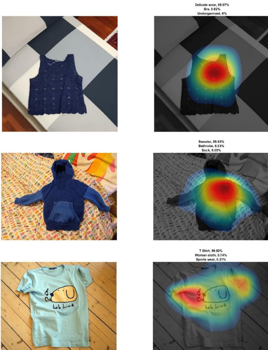
Figure 46. Class Activation Map applied to three images randomly chosen from the database. On the left the original image, on the right the CAM applied to the picture, with the top-3 class predicted by the network.
