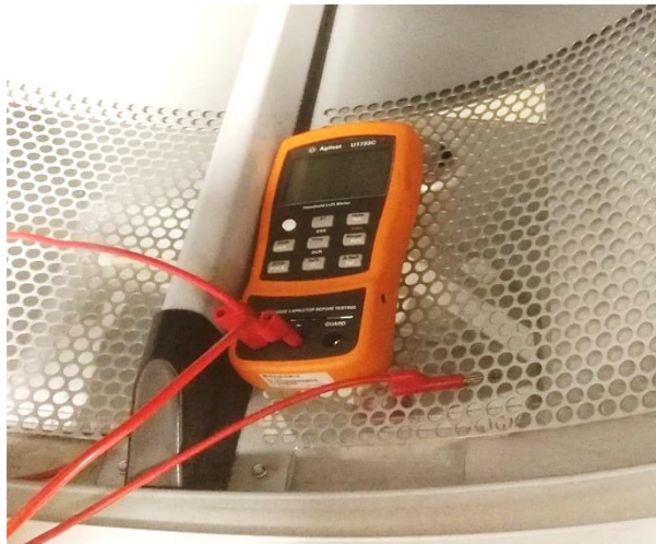
Figure 68. Capacitive meter Agilent U1733C connected to the lifter and to the drum.
