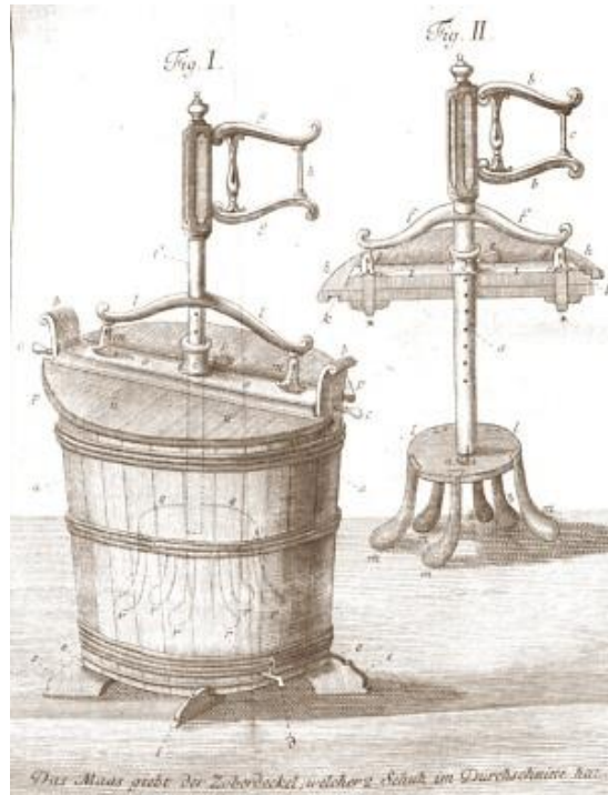
Figure 2. First washing mechanism created by Jacob Christian Schäffer [3].
