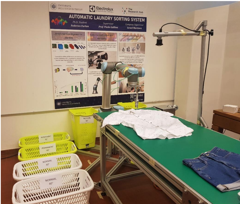
Figure 54. Robotic sorting system in an indoor environment. The baskets are placed around the cobot, that grabs the items onto a conveyor belt. There is one basket for every washing program presented in 2.5. The only sensor used is a camera.
