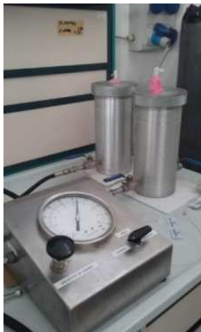
Fig. 1. The modified Sholander pressure chamber used for extracting olive xylem sap.
