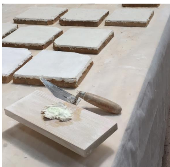
Figure 5. Freshly-prepared marmorino coated-brick.
