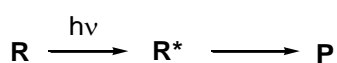
Figure 4. Reaction scheme of a photochemical reaction. R = reagent; R* = reagent in the excited state; P = product; h\nu = light.
