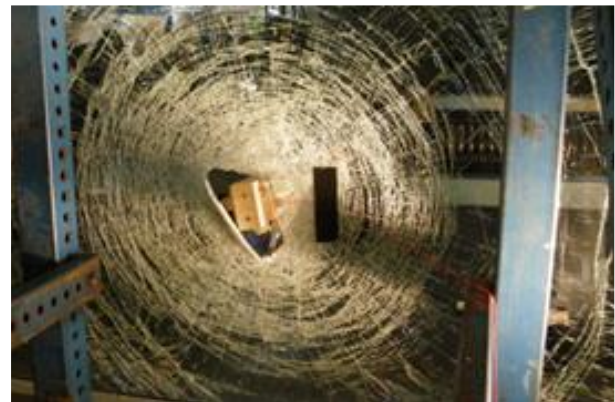
Fig. 1: Damage of laminated glass windows under windborne debris impact
