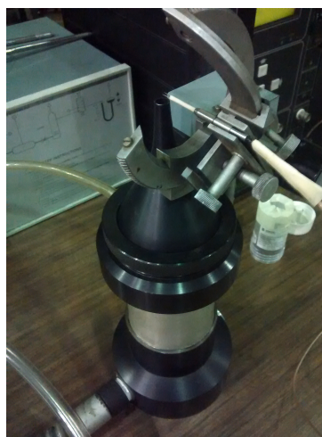
(b) The convergent nozzle and the anemometer wire
