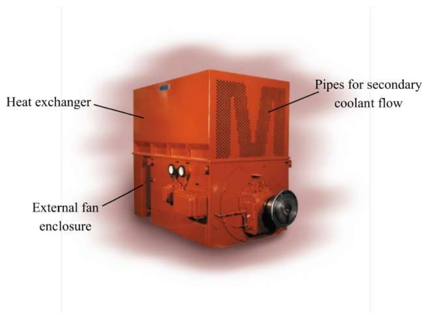
Figure 2.12: Example of a medium-voltage rotating machine with IC611 cooling system. The machine is totally enclosed and equipped with an air-to-air heat exchanger mounted on its top. Forced circulation through shaft-mounted fans is used for both primary and secondary cooling air.
