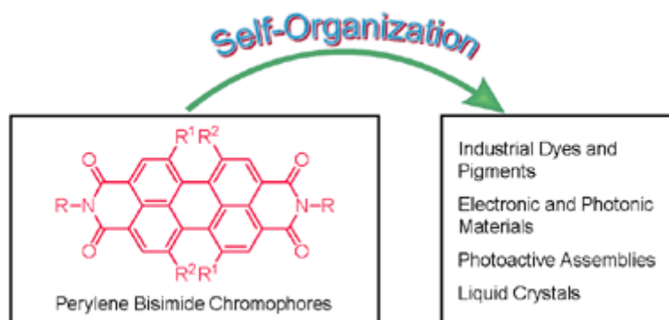
Figure 8. Perylene structure and reactive areas of the compound. Some of the uses of perylene derivatives due to their self-organization properties. 45
